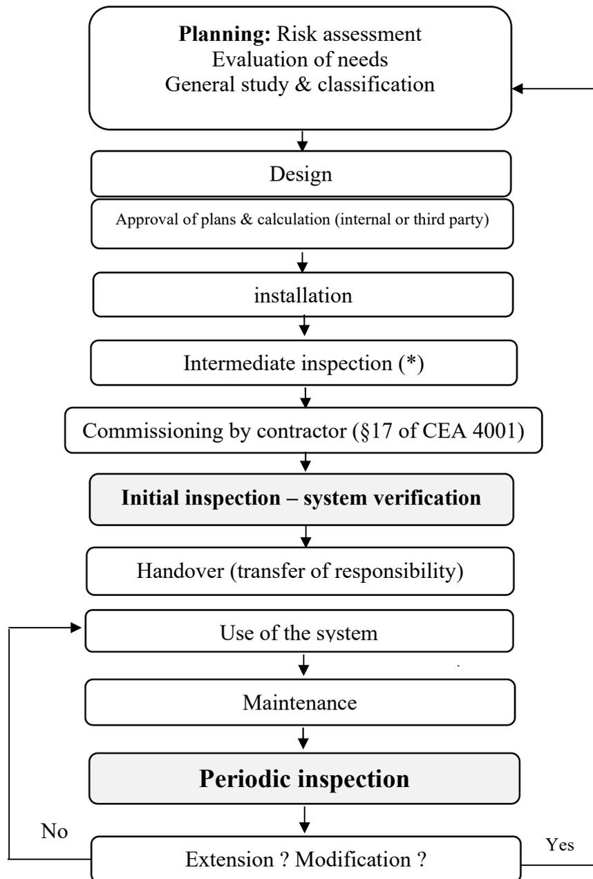
**Figure F 2 — Typical life cycle of automatic firefighting system**
